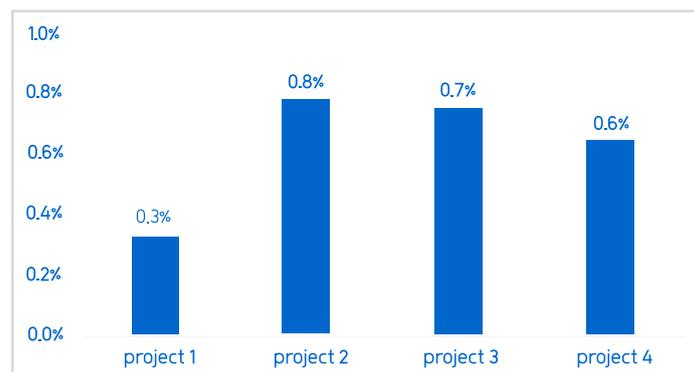
The membrane cleaning and flushing has a weight of (0.62%) of the total capital cost of SWRO desalination plant. One of the lowest cost elements that impact the capital cost, however it has a great role of ensuring and keeping the full life span of the membrane’s equipment.
