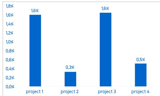
Within the total capital cost of a SWRO desalination plant, the product water pumping station represents a relatively small portion, with a weighted average of approximately (0.97%). Despite its low contribution, this component is vital in facilitating the distribution and transportation of the desalinated water to its intended destination.
