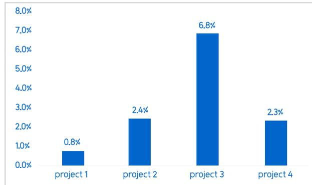
The total average weight of capital cost of the outfall is (2.8%), as the intake the outfall cost varies in relation with structure and the distance of the intake and the outfalls from the seawater.
