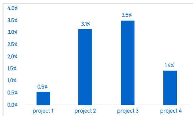
The total average weight of the capital cost of the HVAC is (2.1%). The cost's weight change depends on the size of the building's constructions and the complication of the air flow inside the constructions.
